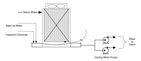
Figure A.3.3 shows a forced draft cooling tower. Warm water from the users enters at the top of the tower then flows down the packing into the basin. Air is pulled into the base of the tower by the fans at the top of the tower. The air flows counter-currently against the warm water. Some of the air evaporates, thus cooling the water. The cooled water is pumped to the users by the cooling water pumps. Make up water and treatment chemicals are added as shown.
