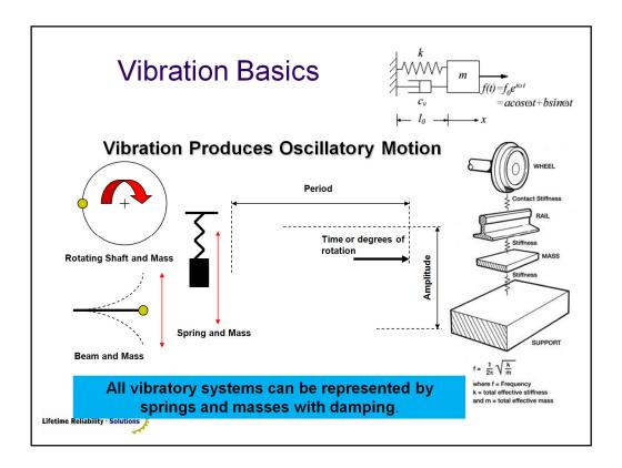
With rotating equipment it is important to have a good appreciation of the causes of vibration.
