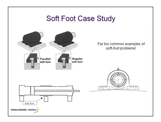
These are common situations where soft-foot occurs. If the items are bolted down without fixing their soft-foot problem, the equipment is distorted out-of-shape, or the mounting feet do not fully contact the base and properly support the forces created when the equipment is used.
